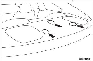
In compliance with the Federal Motor Vehicle Safety Standards, your vehicle has 3 attachment points on the rear shelf, located behind the top of your rear seat. For securing a child seat tether strap to each of the 3 rear seating positions (2 outer and 1 center) in your vehicle.
